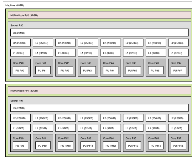
Fig. 1. Architecture topology of an eight-core Intel Sandy Bridge EP dual processor
